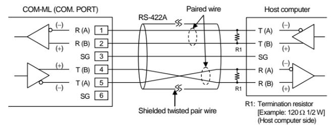
If communication errors occur frequently due to the operation environment or the communication distance, connect termination resistors to the host computer side.
