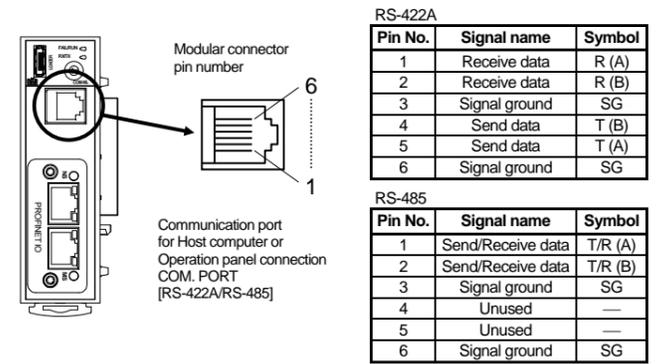
The six-pin type modular connector should be used for the connection to the COM-ML. (Recommended manufacturer and model: Hirose Electric, TM4P-66P)
