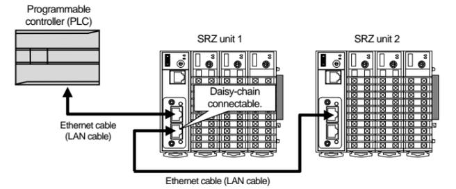
Ethernet straight through cable and Ethernet crossover cable may be used. Ethernet cable (LAN cable) uses category 5 or higher.
