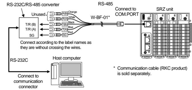
Be sure to insulate the wires that are not used by covering them with insulating tape.
