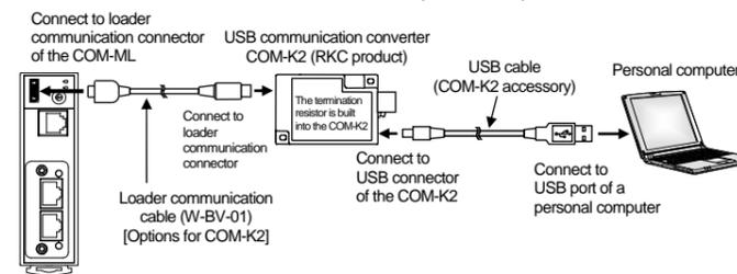
The module address for loader communication is fixed at "0."
